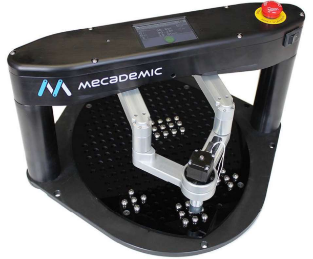
Figure 7: DexTAR (Dextrous Twin-Arm Robot) - Three-Axis Dual-Arm SCARA Robot for Education and Training[6]
