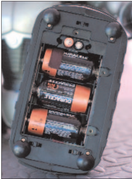
Figure 2. One of the battery compartments. Note the two "AAA" cells at the top.
