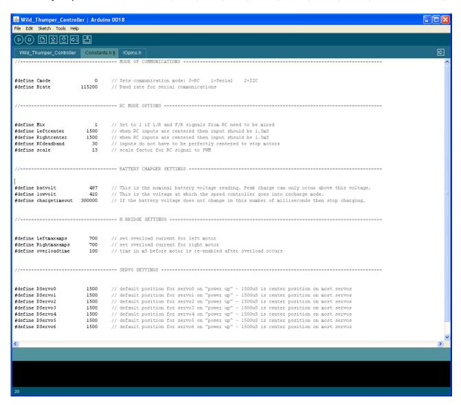
The supplied software is programmed for a 7.2V NiCd or NiMh Sub C battery pack and will need changing if other batteries are used. **Do not use LiPo or Li-ion batteries with this charger!** If you are not sure what batteries you are using then do not use the recharge feature on this board.
