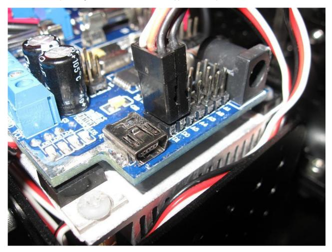
If your battery voltage gets too low (approximately 6V) then the controller will shut down to prevent malfunction and the battery charging circuit will turn on. With a DC voltage of 3-6V higher than your battery nominal voltage applied to the recharge socket your battery will begin charging until the voltage levels out for more than 5 minutes or peaks (delta V) at this point the charger will change to a trickle mode until external power is disconnected.
