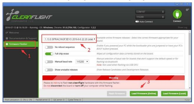
3. Click "Flash Firmware" and wait the ST DFU DRIVER Automatic installation. It's successfully installed when you see the DFU port on the Up right corner.
