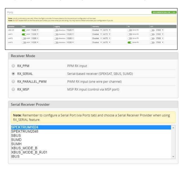
2. For SBUS receiver's soldered to the UART2 GND, + 5V, RX2. Then Enable Serial RX and Set Receiver mode RX\_SERIAL, Select Sbus signal in
