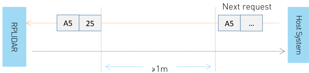
Figure 4-2 The Timing Sequence of a STOP Request
